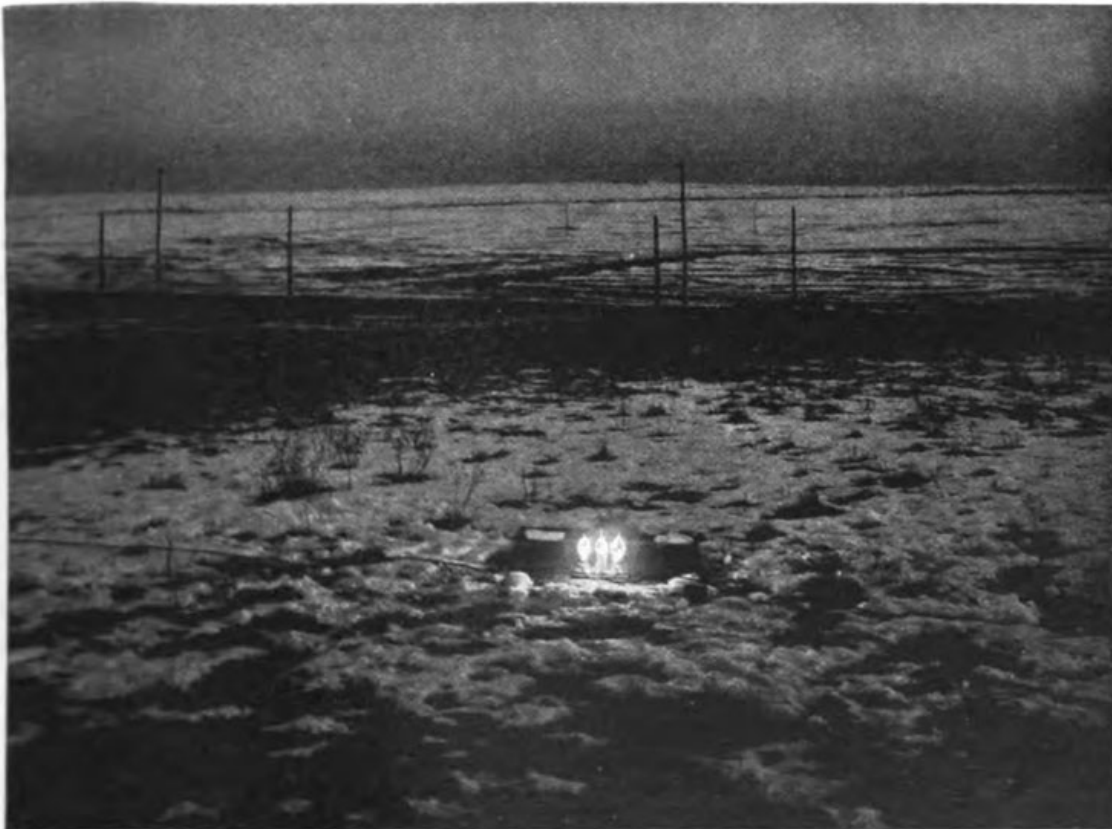
FIG. 7. EXPERIMENT TO ILLUSTRATE AN INDUCTIVE EFFECT OF AN ELECTRICAL OSCILLATOR OF GREAT POWER.
