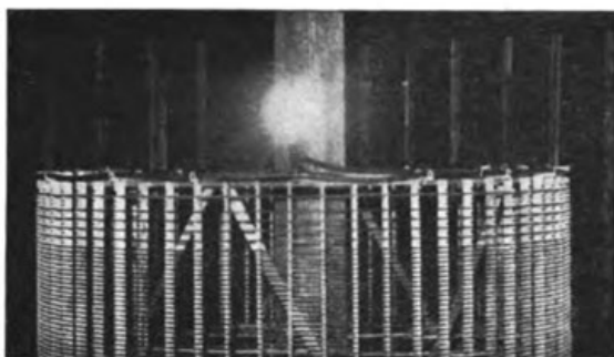
FIG. 3. EXPERIMENT TO ILLUSTRATE THE SUPPLYING OF ELECTRICAL ENERGY THROUGH A SINGLE WIRE WITHOUT RETURN.
