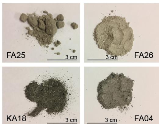
Different texture of fly (FA25, FA26, FA04) and boiler ash (KA18).
