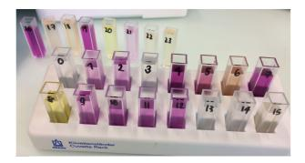
Cuvettes ready to measure with photospectrometric method. Notebthe different color than red-violet (e.g. Nr. 6 and Nr. 8 vs. Nr.9-12), the latter showing the expected red-violet color. Other colors are indications of Cr transitions reactions or interferences. Samples with Cr(VI) concentrations below detection limit remain colorless (e.g. Nr. 3)
