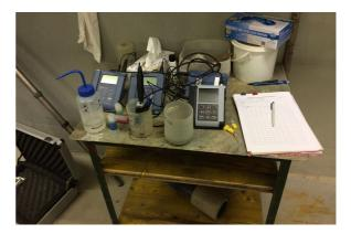
Setup during on-site experiment: monitoring of pH, Eh, O2 during mixed (fly and wood ash) FLUWA with addition of H2O2  $\,$
