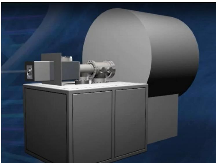
I will shortly comment on the YouTube vides: The video shows a typical ICR mass spectrometer. It is a relatively large instrument with a large magnet. The ions are generated by electrospray ionization. You have learned about the technique, so you know that we generate protonated or multiply protonated ions.
