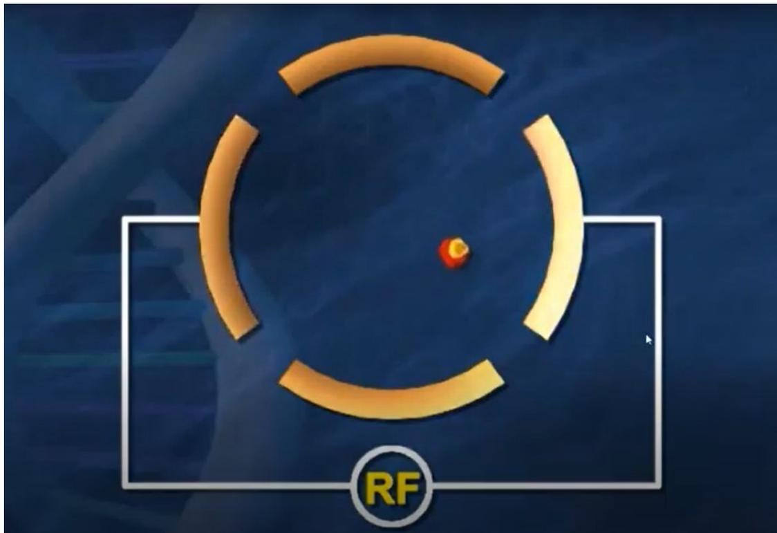
Then we switch off the emitting field and let the ions freely circulate in the magnetic field. We “listen” to the ions by recording the RF current that they generate at the receiver plates. The ions circulate at their typical cyclotron resonance frequencies that are dependent on their mass to charge ratio.
