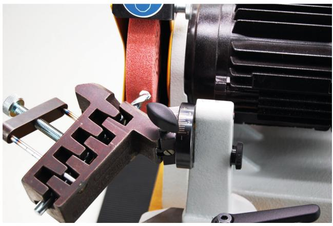
Grinding of **carbide drills** depending on shape of cutting edge use the **4 facet shape** or **twist drills**.
