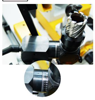
Turn the core drill support to 90° (see picture above).
