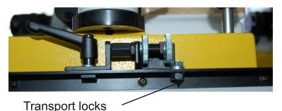
After you have unpacked the machine, remove the transport locks. (see picture)
