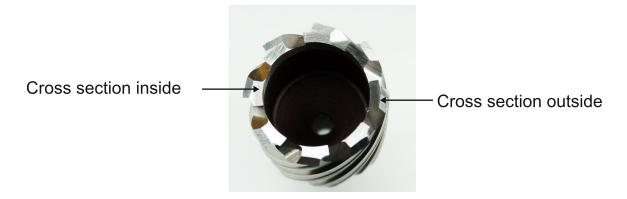
Place the scale of the pillar to **70**° (see picture on page 13) The core-drill support place to **7,5**°
