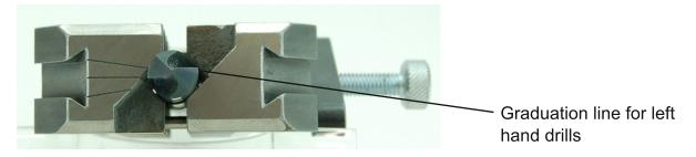
Adjust the requested clearance angle on the scale (Picture below).
