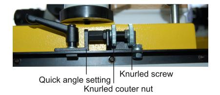
After you have sharpened the first tooth, move back the slide and turn the star knob screw, clockwise up to the next index of the index plate. Do not work with the motor feed.
