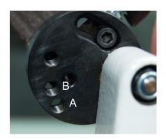
Turning mechanism fix in hole **A**.
