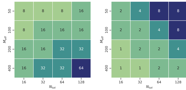
Figure 9: Optimal distribution of resources for different combinations of M_{\text{eff}} and N_{\text{tot}} . Left: Optimal number of parallel chains. Right: Optimal number of threads for prefetching.
