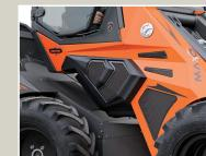
Covered air conditioning system in shockproof material and integrated into the bodywork.
