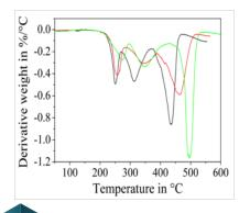
Thermogravimetric analysis (TGA) allows the determination of mass changes of a specimen in dependency of temperature and time. The analysis may be conducted under air or inert gas flow (nitrogen/argon). We can determine:
