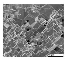
The essentail challenge within plastic-metal-junctions is depicted by the interface which in principle inhibits the formation of strong bonding. With our novel surface-structuring method, we are able to increase the mechanical stability of these junctions many times by mechanical interlocking. We offer:
