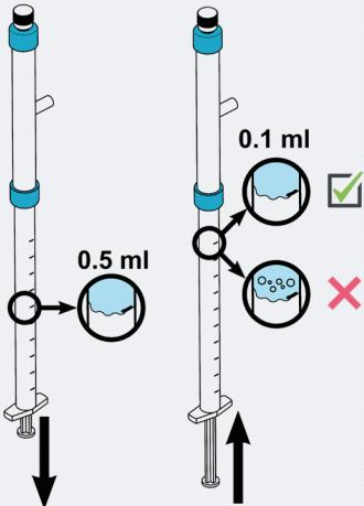
**EN:** Pull the syringe back to the 0.5ml mark. Push the plunger in slowly to the 0.1ml mark to collect 0.1ml of sample exactly.
