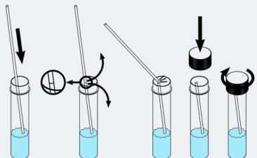
**EN:** Insert swab into the recovery buffer vial. Snap off the swab handle carefully and replace lid.
