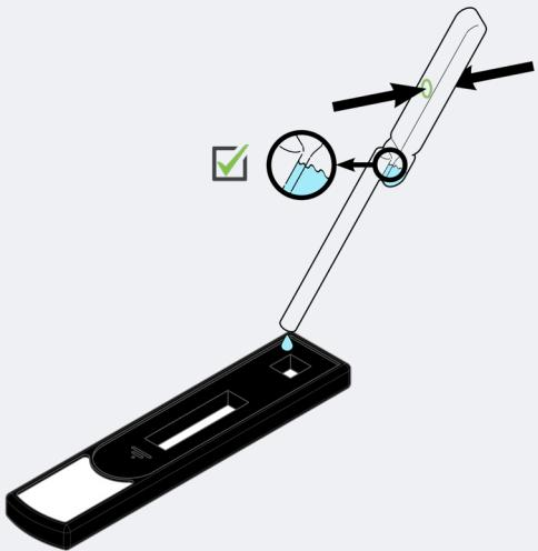
**EN:** Press the top bulb on the pipette to release 0.1ml of sample onto the sample window of the test strip.
