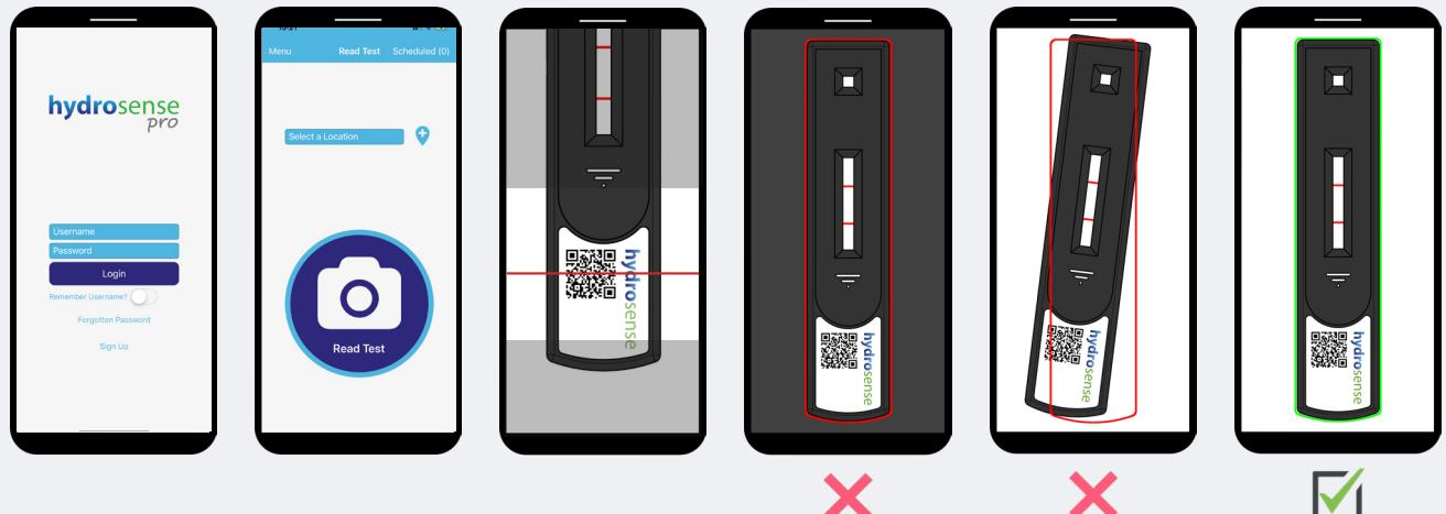
**EN:** Select a pre-programmed location and click read test. Scan the barcode. The scanner will appear on screen. Read the test by matching up the outline of the Hydrosense test on the screen with the cassette.
