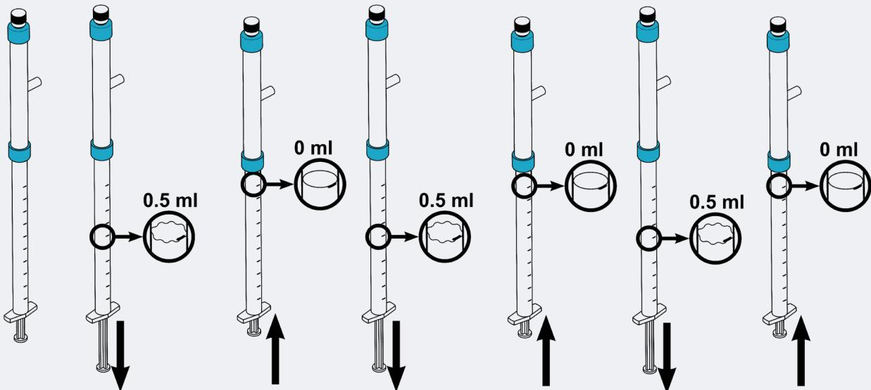
**EN:** Pull the syringe back to the 0.5ml mark. Push the liquid all the way back into the filter. Repeat this step 2 more times.
