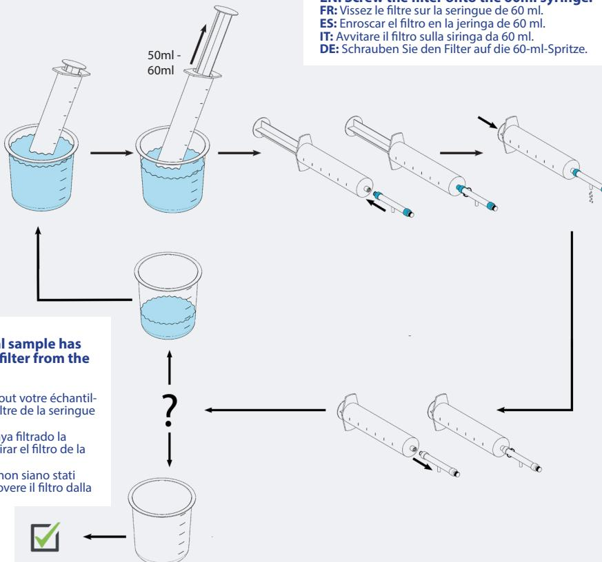
**EN:** Screw the filter onto the 60ml syringe.
