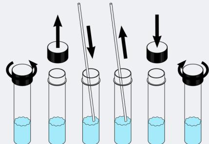
**EN: If testing a dry surface, pre-moisten the swab by dipping it into the recovery buffer vial.**
