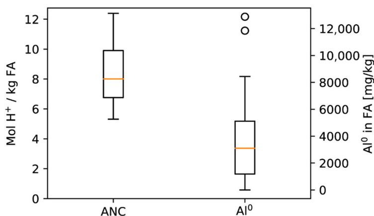
**Figure 4.** Boxplot of the acid neutralizing capacity (ANC) as amount mol H<sup>+</sup> to reach pH 2 at a L/S ratio of 10 and Al<sup>0</sup> in Swiss FA (n = 29).
