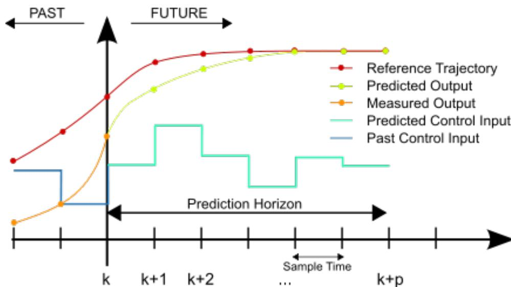
Figure 4. Model predictive control featuring a moving prediction horizon.
