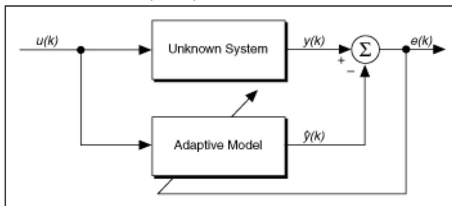
Figure 2. Example of system identification input  $u$  and output  $y$  are used to minimize the error  $e$  between  $y$  and model output  $\hat{y}$ .
