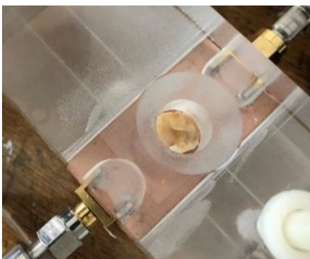
Figure 8. Sample holder setup with an atheromatous plaque
