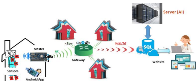
Figure 3. Overall architecture of the proposed sleep monitoring system
