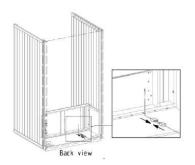
No.1: Connect the plug of the bench heater to connector A and make sure they are tightly connected.
