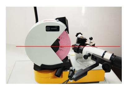
Fix the support plate of the **BSG 60** with the star knob screw in boring hole **A**. The stepless clearance angle adjustment has to be turned to scale value **2**.
