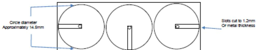
Perform all precision cut work before separating the components.
