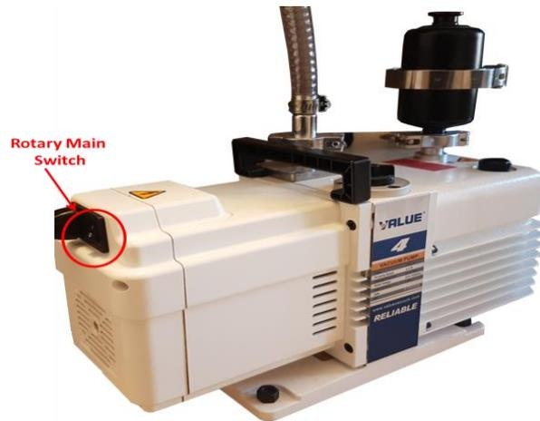
Figure 5-1: Main switch of the backing pump
