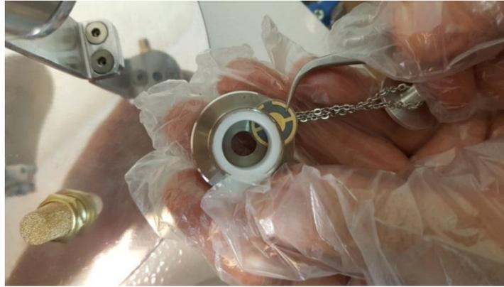
Figure 6-3: Insertion of new crystal to the groove
