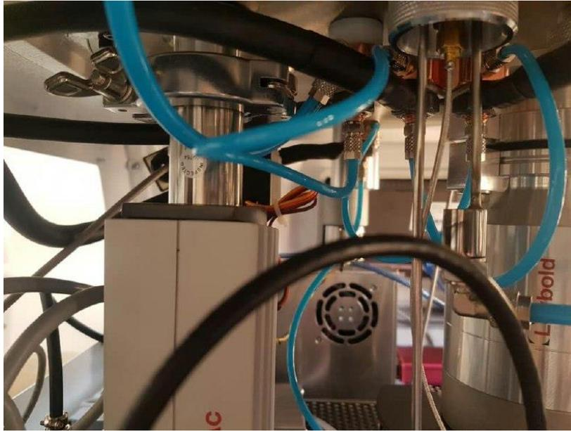
Figure 3-6: Feedthrough and thickness meter cooling system (Plastic blue hoses)
