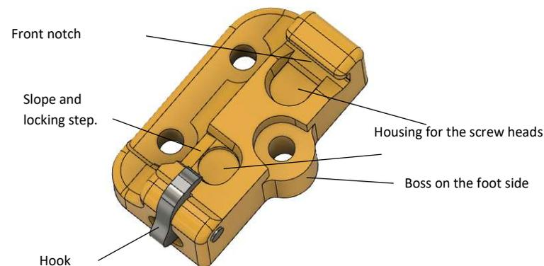
**Mounting the supports:** The 2 parts are symmetrical. The hook must be located towards the heel, the boss for the screw on the foot side being lodged in the hollow of the arch of the foot. The part shown above is suitable for the right foot.
