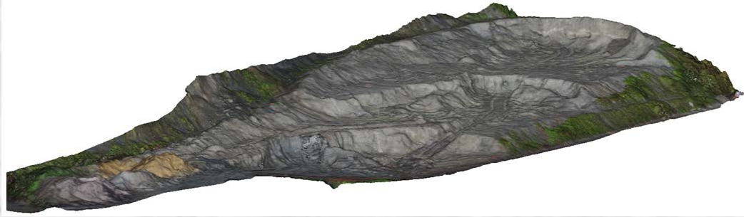
Digital surface model - stockpile cubature
