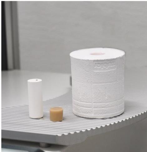
ingot, single-use plunger and muffle
