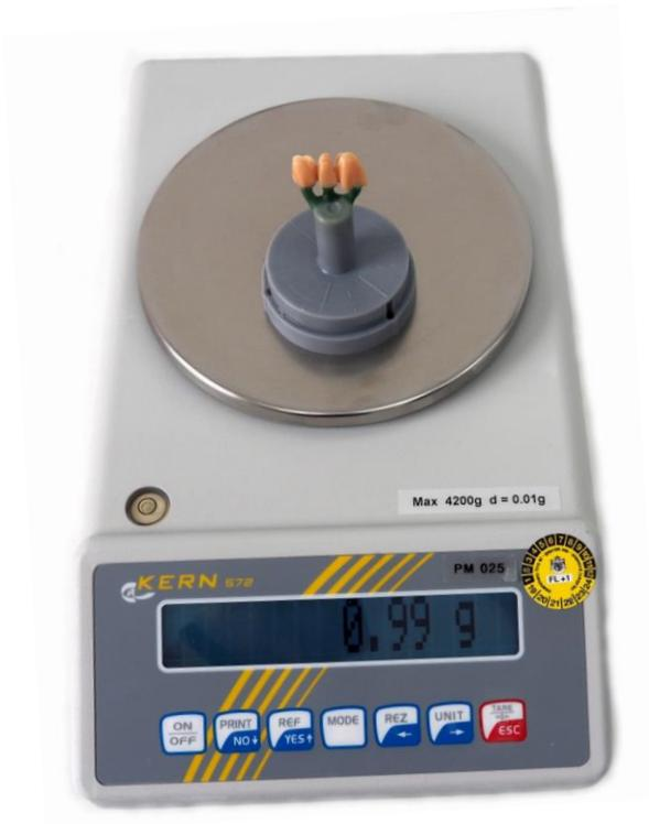
**Note:** Weigh the empty press base - then weigh the press base with the respective modeled object.
