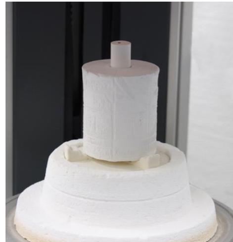
Muffle in pressing furnace
