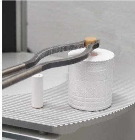
Place the ingot into the muffle
