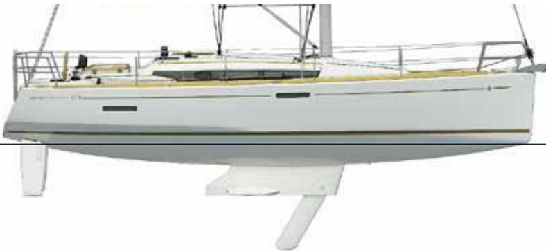
The advanced winged keel, for the swing version, provides more performance thanks to a lower centre of gravity and better upwind performance, with the possibility of sailing in shallow waters.
