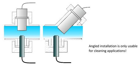
The drawing is symbolic of all installation situations and differs according to the connection fitting.
