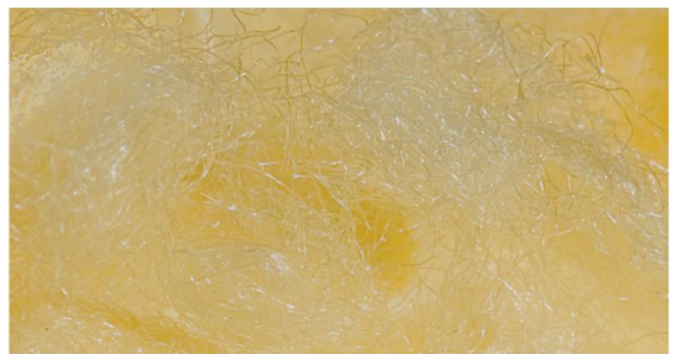
Aqualen™ ion-exchange fiber Fiber diameter: 10 microns Surface area: 1000 cm 2 /g
