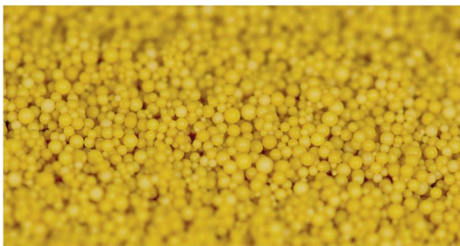
Conventional ion-exchange Granule diameter: 700 microns Surface area: 10 cm 2 /g
