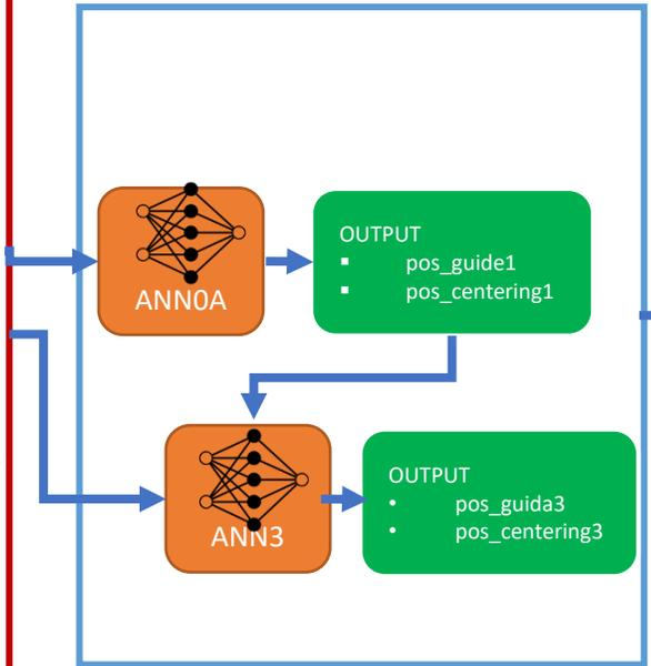
❖ Calculation of index on each position of coil length based on the value of guide and centering device predicted by ML model
