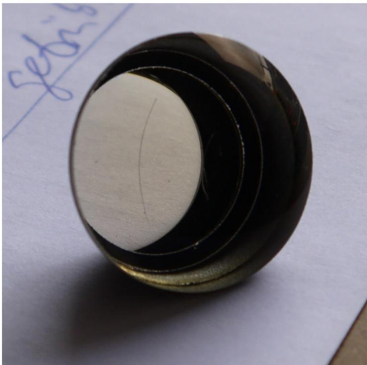
Here is a view of a cemented doublet from the finder optics of an Arriflex 16. A hair seems to be trapped, yet it has turned out to be a step within the resin. I take pride in being able to separate such groups and renew the bond with Canada balsam or synthetic compounds.
