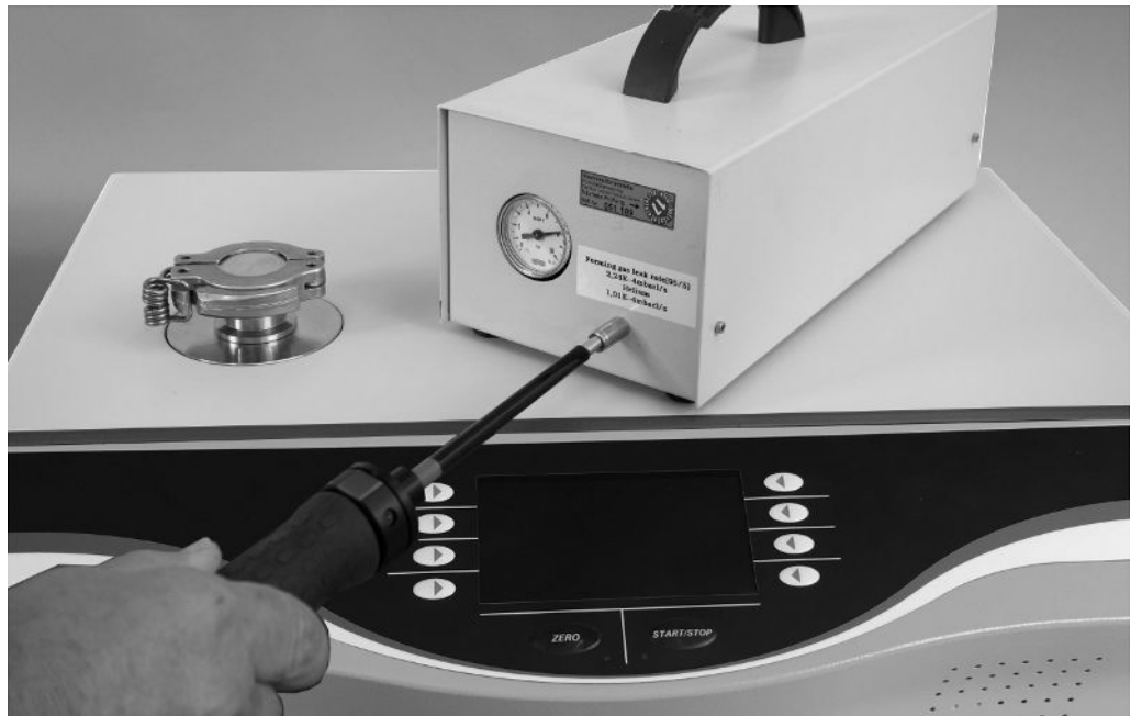
Fig. 17: Sniff test on an external calibration leak
