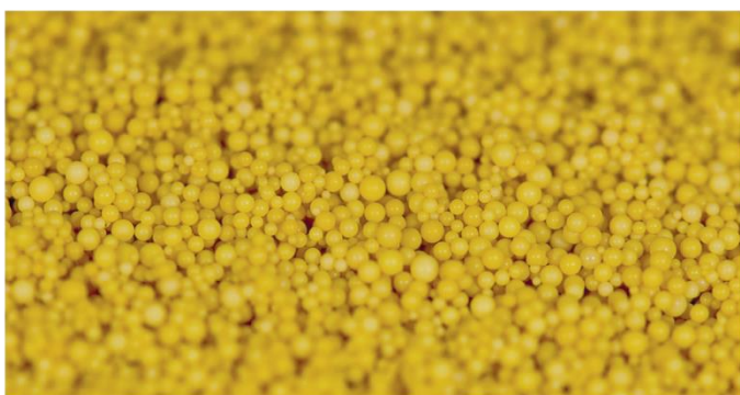
Conventional ion-exchange Granule diameter: 700 microns Surface area: 10 cm 2 /g
