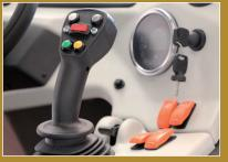
Electronic display with warning lights Joystick 5 and 11 functions. Maximum speed : indicating faults, engine, hydraulic 11-functions Joystick is standard on 12 Kmh LX models.
