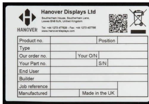
Figure 3a – silver label (pre July 2022) on casing of destination controller
