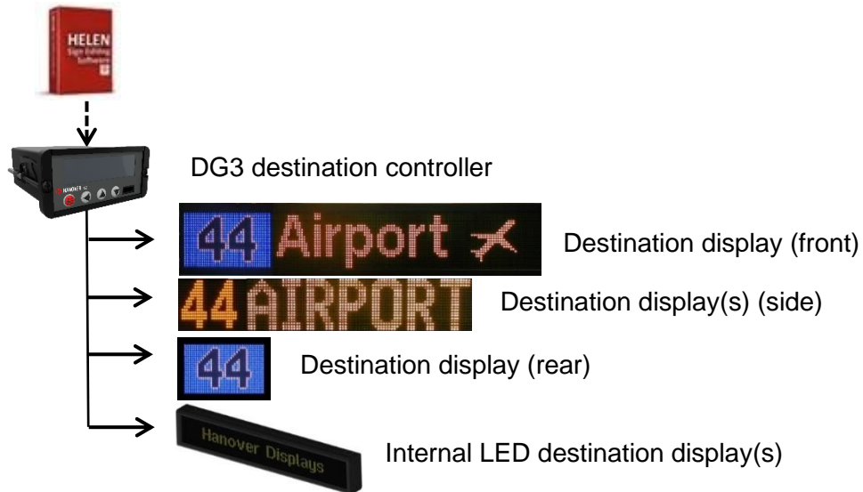
Figure 1 - diagram showing typical destination controller / displays configuration. Each unit is powered individually.
