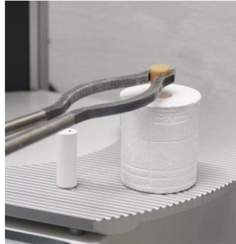
Place the ingot into the muffle
