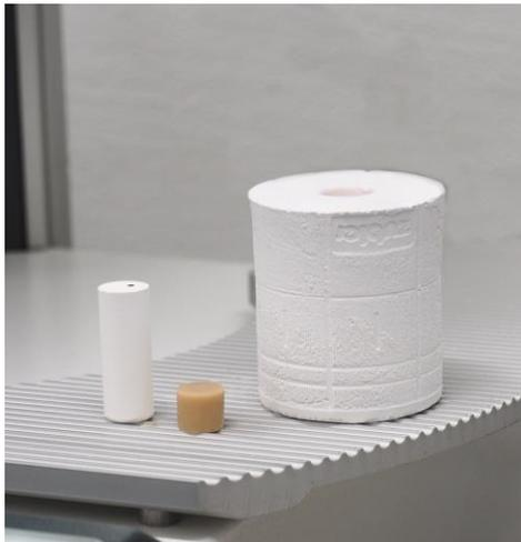
ingot, single-use plunger and muffle
