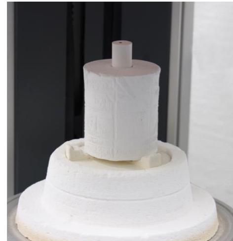
Muffle in pressing furnace
