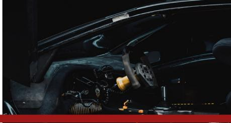
Driver safety is one of the most important things when it comes to building a racecar and required to attend in official racing series. That's why the REITER Diablo is equipped with features such as an integraded roll cage, fire extinguisher system and safety fuel cell, Also a REITER manufactured, FIA certificated driver seat is installed.
