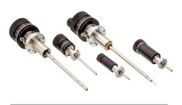
The RD1 is a low backlash, high precision edge welded bellows drive providing continuous primary rotation to a 9.52 mm diameter shaft.
