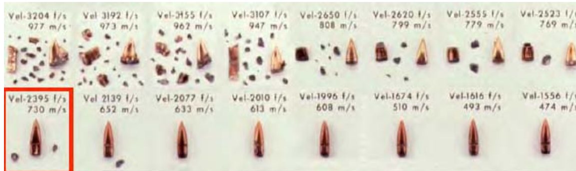
Figure 1. 5.56-mm fragmentation at various velocities. Below 2,500 feet per second, fragmentation does not occur. Source: http://www.dtic.mil/ndia/2008intl/Roberts.pdf (accessed March 25, 2009).
