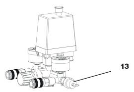
The safety valve is incorporated into the pressure switch unit, the safety valve opens if the max, permissible pressure is exceeded, Will be not accepted adjustment
