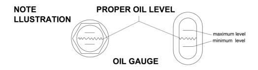
\*The lubricant oil should be of oilness and contain inhibitor, not easy to be oxidized, get densified or foamed, low residual carbon, hight flash point.
