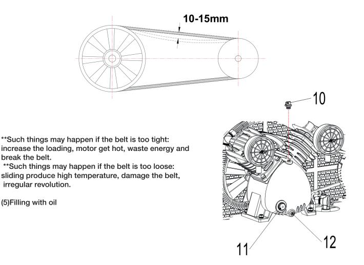
Remove the oil plug (10) Fill with oil up to the centre of the level indicator(11) Install back the oil plug(10)
