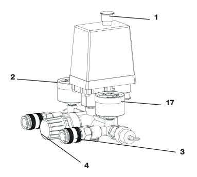
2. Set pressure regulator(4)to required working pressure. The current working pressure is indicated by the regulated pressure gauge(17).
