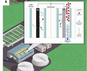
Figure 1. Schematic illustrating photoelectrochemical systems (A) Commonly tested batch-mode systems at the bench scale. (B) Representative flow system for full-scale treatment applications.
