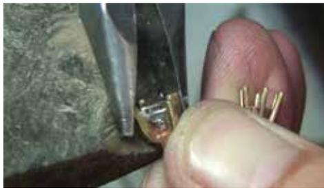
**9** Constantly check the level of the stone and the positioning of the claws.
