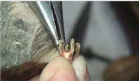
**8** You can use a pushing tool to move the claw tips onto the crown facets. Each claw should be pushed a little at a time on opposite sides, this technique will keep the stone level.
