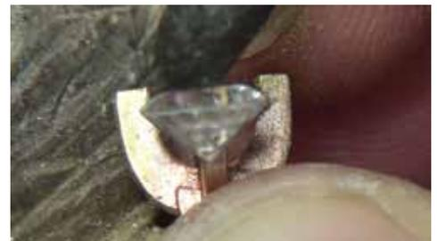
**7** If you are working on a project or a commission, ensure the setting is prepared for a final polish before the stone is placed.
