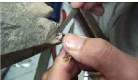
**11** Jewellers generally need to make specialised tools for certain tasks. For the final forming of the claw tips, use a steel pusher with a 'V' shape cut into the end. This can be used to push and burnish the open edge of the tip until it closes fully onto the stone. It also hardens the tip for longevity.
