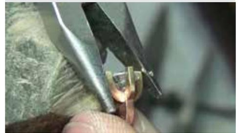
**10** The claw tips can now be trimmed down and shaped with a needle file. Ensure the file has a safety edge to limit stone damage.
