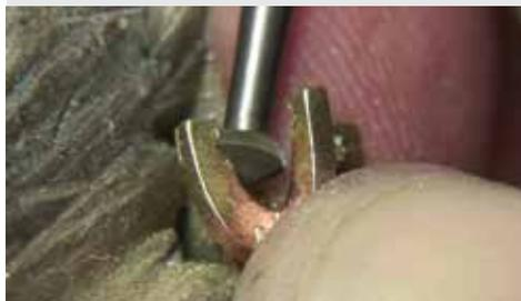
**6** Check to see if the cut matches the profile of the stone. Examine the girdle of the stone you are setting. If it is thick then you will need to adjust the seating cut with a fine tapered bur to match the girdle thickness.
