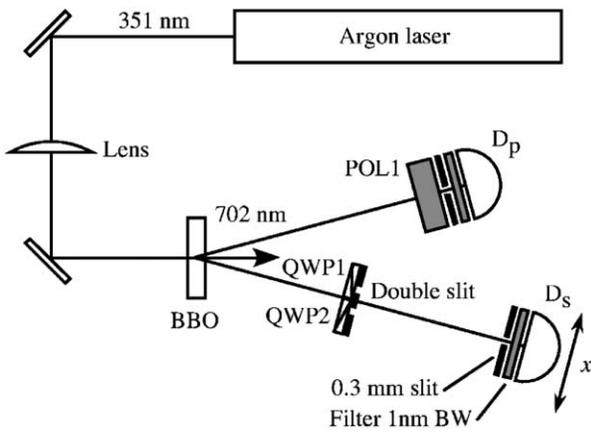
FIG. 8. Setup of the quantum eraser experiment of Walborn *et al.* (Ref. 14).
