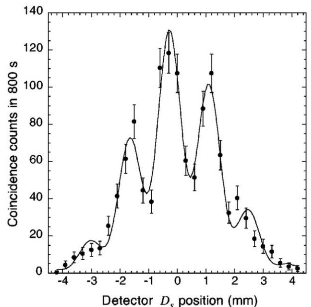
FIG. 11. Coincidence counts when QWP1, QWP2, and POL1 are in place. POL1 was set to  $\theta$ , the angle of the fast axis of QWP1. “Interference has been restored” in the fringe pattern (Ref. 14).
