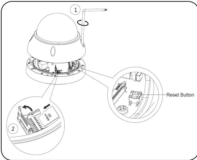
**Note:** For reset (used to return the camera settings to factory default mode), long press the Reset button for 8 seconds; the light turns off.
