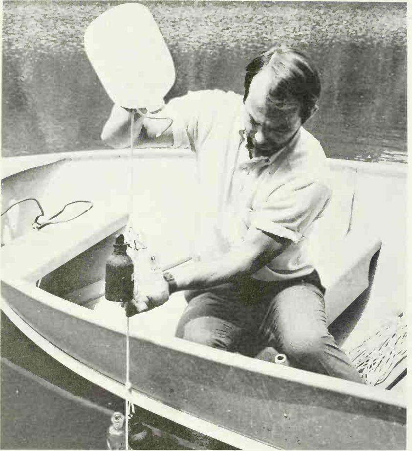
Fig. 2-4 Measuring the metabolism of a pond by the light-and-dark bottle method. Pairs of black and transparent bottles are lowered into position, while the plastic jug acts as a float to hold the pairs at the desired levels for measurement of oxygen changes. See text for explanation.
