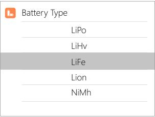
The charger supports charging and discharging of 6 types of batteries: Lipo, LiHV, LiFe, Lion, NiMh, and PB. And two modes of power supply and the smart battery
