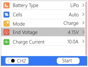
Move the cursor to [Battery Type] and press [OK] to modify the battery type, as shown below:
