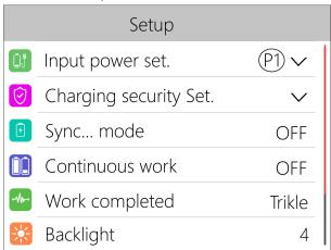
**Input power settings:** Enter the relevant settings of the power supply. After long-pressing, can select power supply 1, power supply 2, and power supply 3. Short press to expand settings. As shown below.
