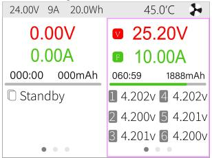
Rotate the [Scroll wheel] on this interface to switch the bottom status information and internal resistance voltage value. Short press [OK] to dynamically set the working current or stop working. As shown below.
