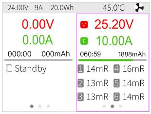
1  $14m\Omega$ : Internal resistance of the first battery
