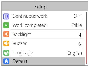
Buzzer: The tone of the buzzer can be set to off.
