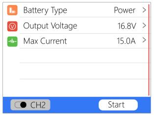
Move the cursor to [Output Voltage] and press [OK] to modify the output voltage. The voltage range is 1V to 28V. Move the cursor to [Max Current] and press [OK] to modify the maximum current, which is the maximum current of the output power supply. The range is 0.5A to 15A.
