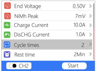
Move the cursor to [Cycle times] and press [OK] to set the cycle times to 2-12. The charger will follow the pattern cycle of discharging-> charging-> discharging-> charging ... "Discharge-> Charge" is 2 times.
