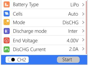
Move the cursor to [Discharge Mode] and press [OK] to modify the discharge mode, as shown below.
