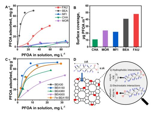
**Fig. 3.** A) PFOA adsorption isotherms; B) PFOA surface coverage on zeolite frameworks; C) Influence of the SiO<sub>2</sub>/Al<sub>2</sub>O<sub>3</sub> ratio on the PFOA adsorption isotherms; D) Hydrophobic interaction between PFOA tail and Si, as well as electrostatic interaction between negatively charged PFOA head and Fe sites on the zeolite surface.
