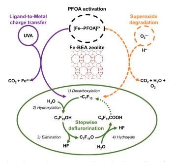
**Fig. 8.** The proposed PFOA activation mechanism through Fe complexation for stepwise DHEH defluorination via ligand-to-metal charge transfer and  $O_2^{-1}$  under UVA initiation. Fe corresponds to the metal and PFOA corresponds to the ligand. The electron transfer occurs from the carboxylic group to Fe<sup>3+</sup> in [Fe-PFOA]<sup>2+</sup>[73]. The orange dotted line suggests the possible involvement of  $O_2^{\bullet-1}$  in the defluorination process.
