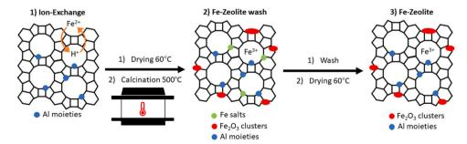
Fig. 1. The scheme of Fe-zeolite synthesis process.
