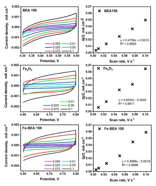
**Fig. 7.** Cyclic voltammetry measurements for BEA150,  $Fe_2O_3$ , and Fe-BEA150 (left); and current density difference ( $\Delta j/2$ ) as a function of the scan rate (values in the colored legend) corresponding oxygen adsorption capacity of the different materials (right).
