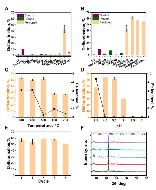
**Fig. 4.** Defluorination of PFOA by A) different zeolite frameworks and B) zeolite BEA with different  $SiO_2/Al_2O_3$  compositions; Defluorination and Fe-leaching at different C) calcination temperature and D) pH by Fe-BEA 150; E) Reusability of Fe-BEA 150; F) XRD diffractogram of Fe-BEA 150 marked BEA characteristic peaks at 7.7 and 22.5° [52] at different calcination temperatures (300–700 °C).
