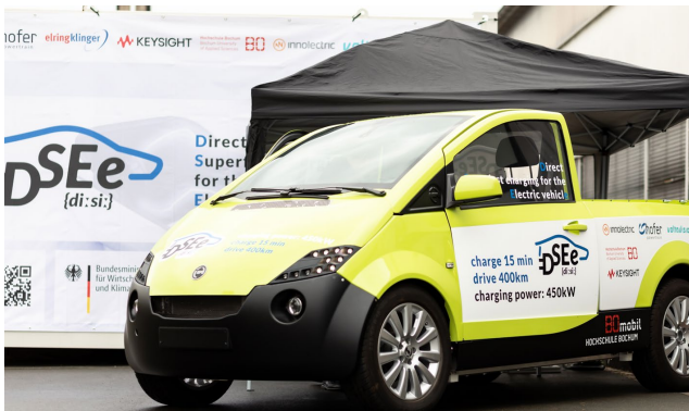
Figure 2: The BOmobil stands in front of the container that contains the charging electronics for the fast charging process.
