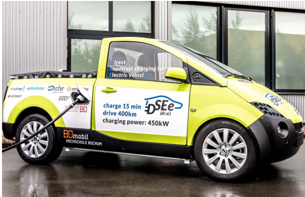
Figure 1: The BOmobil was specially equipped for the "D-SEe" research project with a new and powerful battery to enable fast charging of 15 minutes for a 400 km range.
