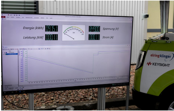
Figure 3: The BOmobil was charged "live" as part of the final presentation of the research project. The exact measured values of the charging process can be read on the monitor.
