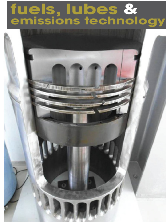
A cutaway of an MAN liner and piston with damage to the piston rings
