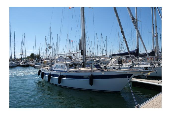
Motiva 39 S, steel yacht, round bilge, semi long keel, Sloop-rigged with pilothouse, center cockpit, warm galvanisation
