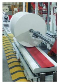
Extra-large reels transport line with different packaging solutions: winding, stretch wrapping, strapping, etc.
