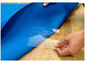
The Circle Cutter comes with a cutting board. Place the cutting board under the canvas where you're about to cut.
