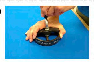
Place the circle cutter over the center of your marked spot. Rotate the knob one full circle to achieve a perfect hole. WARNING: Make sure your other hand is clear of the path of the blade.
