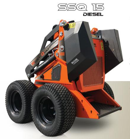
Kubota engine Z602, displacement 599 cc. Number of cylinders: 2 Start: electric RPM: 3200 Cooling: liquid Fuel: Diesel Fuel tank capacity: 25 liters Hydraulic system: 25,6 l/min - 200 bar Hydraulic oil tank capacity: 25 liters Steering: skid Weight: 684 Kg
