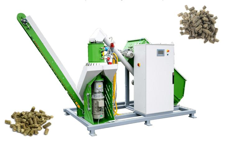
The **press** is avaible in power classes 11/15/30 kW. Different mattresses allow not only different types of matrices. To process raw materials, but also to vary the diameter of the finished pellets and to influence the bulk weight. The presses are equipped with humidity monitoring, temperature monitoring and overfill protection as standard.
