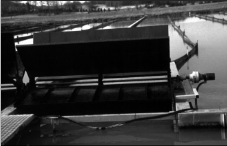
Figure 4. Hydraulic-powered, low-speed paddlewheel used to mix the partitioned aquaculture system. Paddlewheels rotate at 1 to 3 rpm. Photo: John Collier.
