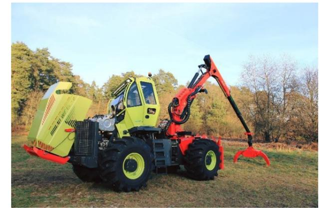
MOTORHAUBE, FRONTSCHUTZ, HYDRAULIKTANK UND KABINE HYDRAULISCH KIPPBAR
