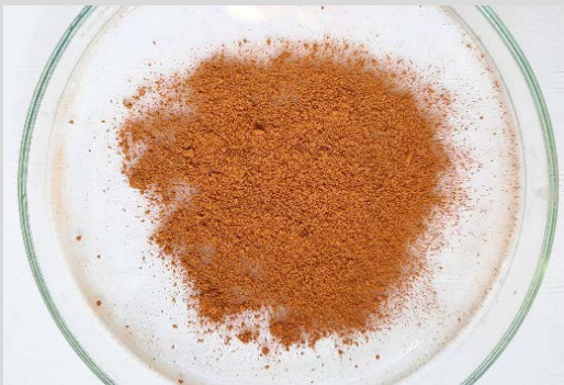
Photo of the schwertmannite synthesized in our lab.
